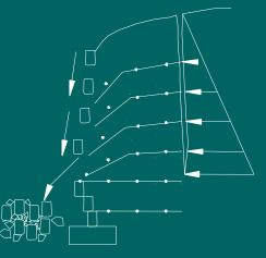
(e) progressively blocks drop along with gravel and some backfill soil
