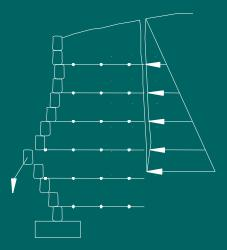
(c) deformation continues; single block dislodges and drop to toe of wall
