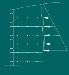
(a) crack forms; water enters and pressure mobilized
